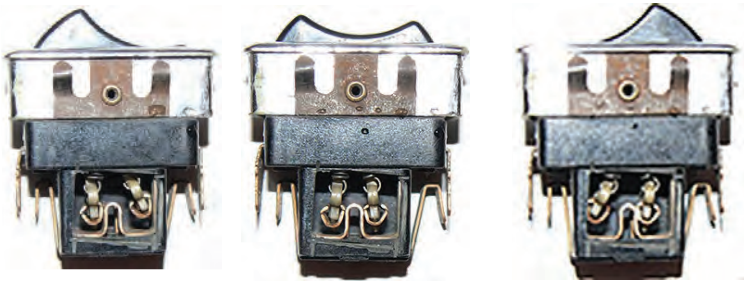
Figure 1 at left, Typical contact numbering. Figure 2 above shows contact connections at three different switch positions. Photos below show a typical switch at each position. The window regulator switches in the Milano would be a good example of this kind of switch.
